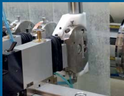
Cut Cleaner installed onto a slitter - non-woven production line
