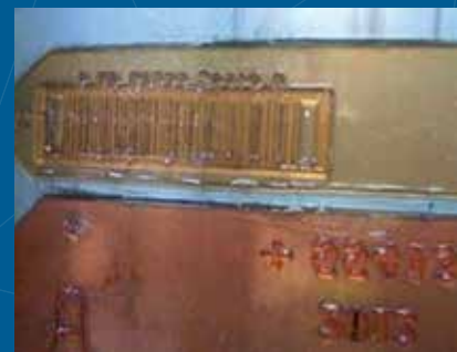
Polymer plate just cleaned from LCV washing machine, ready for storing.
